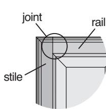
humidity within the home. When these natural dimensional changes occur, joinery lines can appear that were not visible before. For instance: As wood swells and contracts due to seasonal humidity changes, a joint where a stile and rail meet can open up slightly, showing a line that was not previously visible. When exposed to drier air, door center panels
