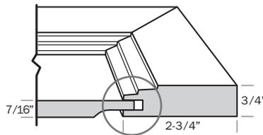
**Paint grade doors use MDF** for the center panel which minimizes expansion and contraction, but joint lines may still appear because paint grade doors have natural wood frames that will expand and contract more than the MDF center panel.
